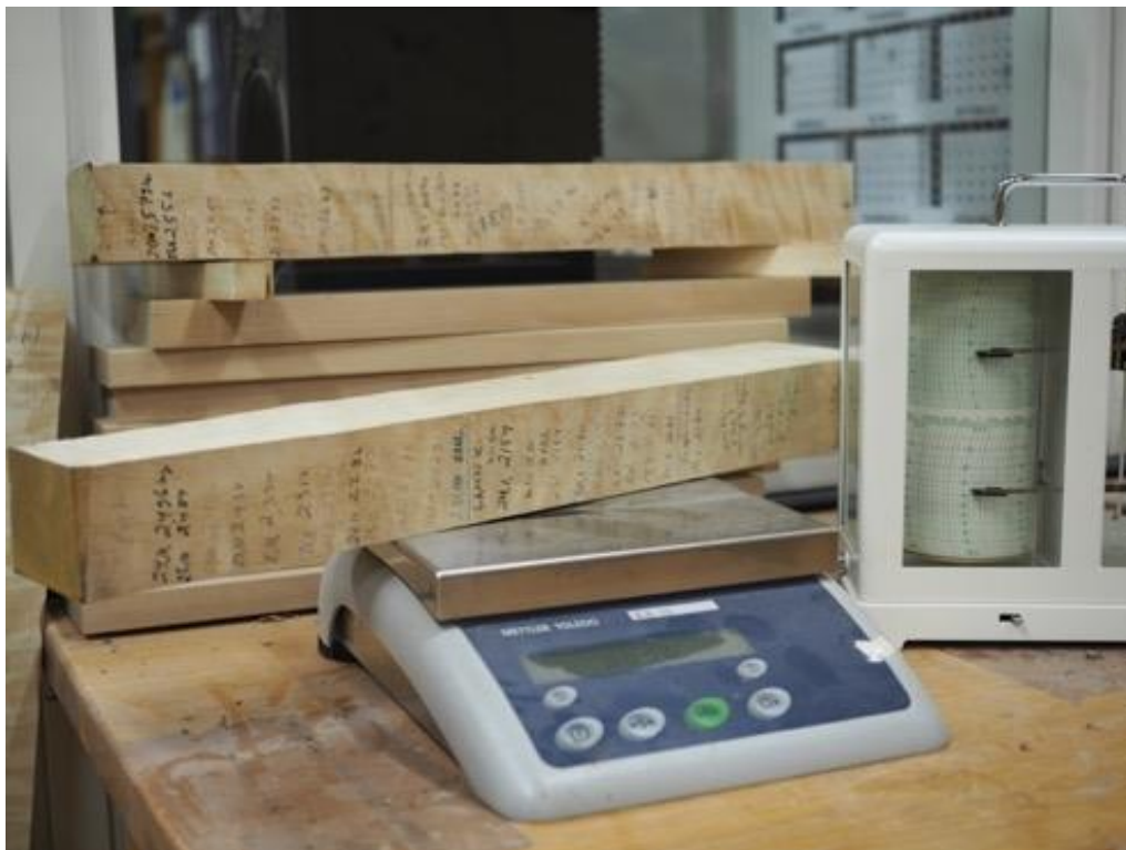
Measuring the equilibrium moisture content with precision scales. The relative humidity of the room is observed with a hygrometer. Photo: Rauno Nieminen
