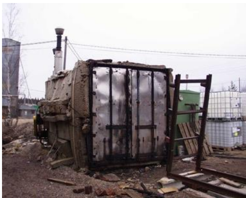
Osmo Savolainen's 1st and 2nd thermal modification ovens in Mänttä. Photo by Rauno Nieminen.
