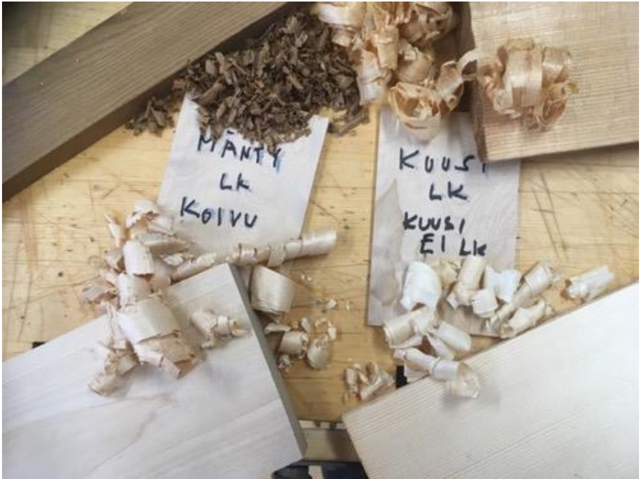
Above pine and spruce treated in too high temperature for musical instrument making. Below thermally aged birch and spruce. Luthiers have many methods to test the wood they use. Common sense takes you a long way.
