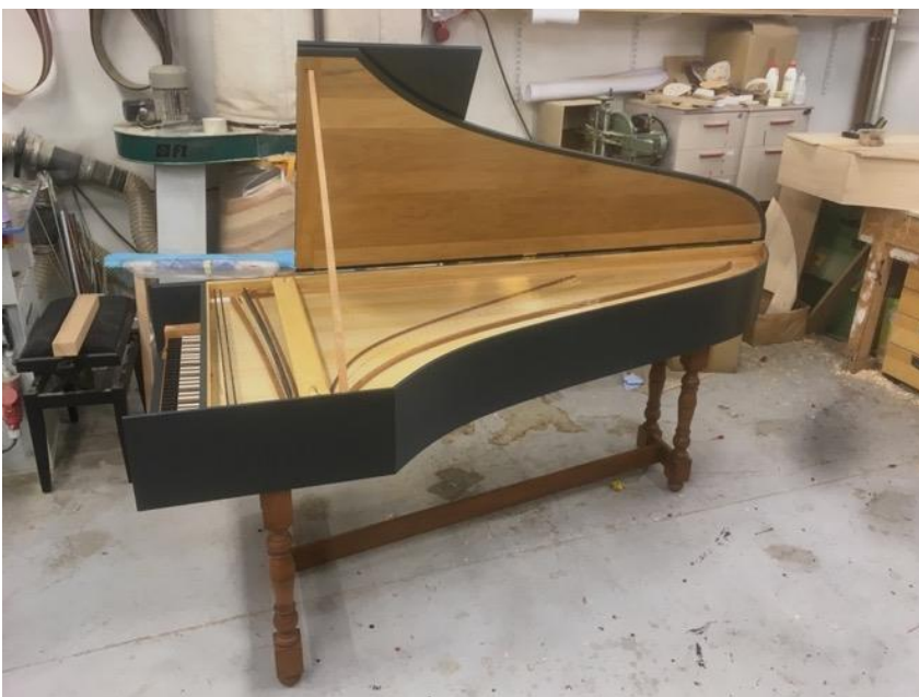
Cembalo made of Thermally Aged Tonewood by Jukka Ollikka. Photo by Jukka Ollikka.
