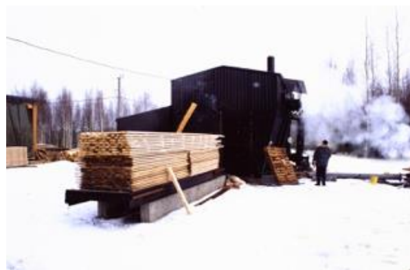
Osmo Savolainen's 1st and 2nd thermal modification ovens in Mänttä. Photo by Rauno Nieminen.
